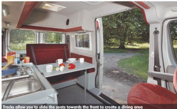
Tracks allow you to slide the seats towards the front to create a dining area
